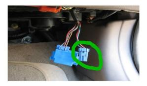
There is no OBD port on the Honda SMX, diagnostics of the ABS Management Light is done via flash codes.
